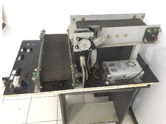
Gambar 2. Alat peraga Apple Conveyor
